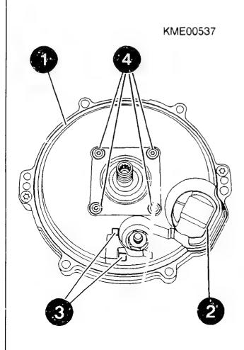
ASSEMBLING ALTERNATOR Sealing alternator Seal alternator at locations indicated. Allow adhesive to run evenly into the grooves until the contact surfaces are properly covered. ATTENTION: Following sealing allow adhesive to cure for 48 hours. Adhesive VS 18295-KK: 5 997 753 000
